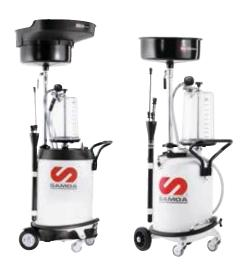
**Combined oil suction and gravity collection units, with transparent chamber.** Units with a 10 liters transparent chamber that can be used as a vacuum reservoir and allows an immediate inspection of the extracted waste oil. They can be used as autonomous units once vacuum is created inside their steel reservoir. Discharge through a discharge hose pressurizing the unit at 0,5 bar using a tire inflator.
