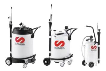
**Oil suction collection units.** They can be used as autonomous units once vacuum is created inside their steel reservoir. Discharge through a discharge hose pressurizing the unit at 0,5 bar using a tire inflator.
