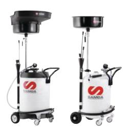
**Combined oil suction and gravity collection units.** They can be used as autonomous units once vacuum is created inside their steel reservoir. Discharge through a discharge hose pressurizing the unit at 0,5 bar using a tire inflator.
