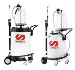
**Oil suction collection units with transparent chamber.** Units include a 10 liters transparent chamber that can be used as a vacuum reservoir and allows an immediate inspection of the extracted waste oil. They can be used as autonomous units once vacuum is created inside their steel reservoir. Discharge through a discharge hose pressurizing the unit at 0,5 bar using a tire inflator.
